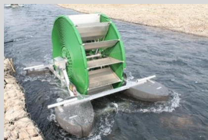
Barsha pump of aQysta at work
