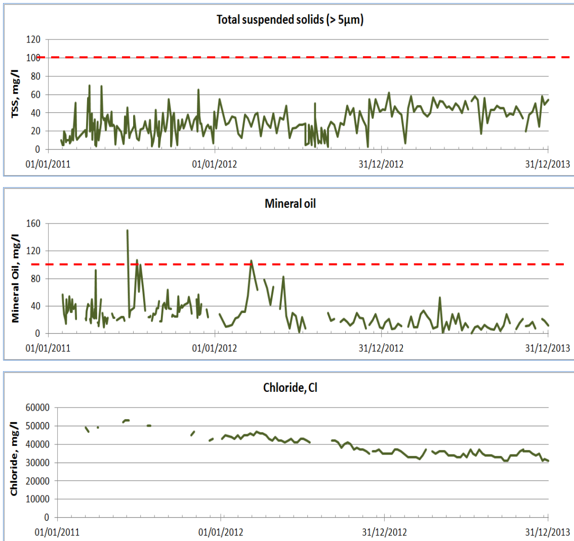
Figure 14 – Suspended solids, oil-in-water and chloride concentrations measured in the injection water at the CTF. The dashed red line indicates the expected max. value. Note that there is no limit for the chloride concentration.
