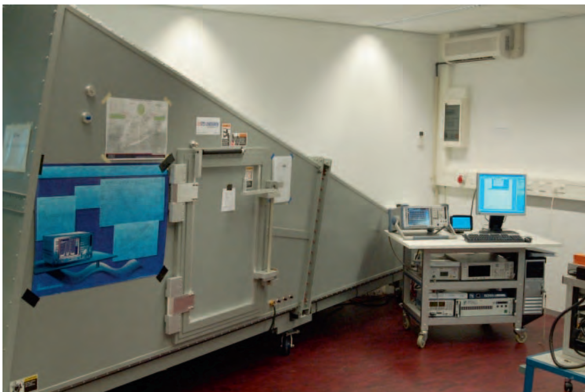
Figuur 3. Meetopstelling immunitieit; GTEM (Gigahertz Transverse Electromagnetic Cell)
