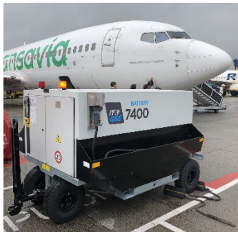
eGPU supplies power to stationary aircraft without emissions
