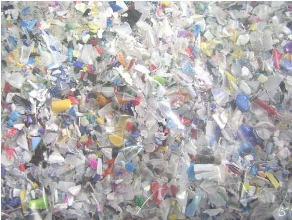
Cleaned polyolefin output from Herbold
