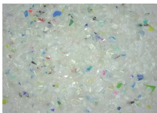
3 rd pass coloured PO flake reject from SEA Srl trial
