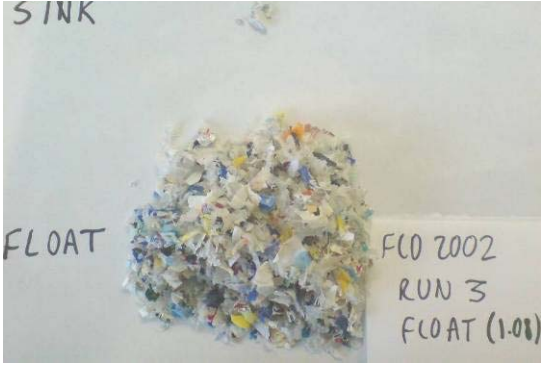
Flottweg float fraction after independent flake testing
