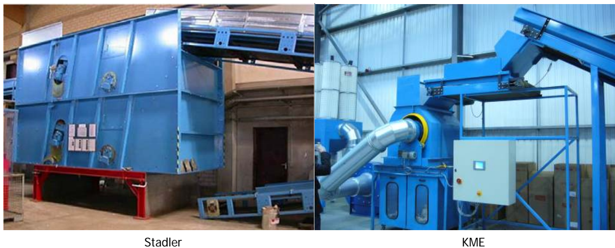
Figure 17 Stadler STT2000 and KME Air Drum Separator
