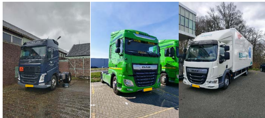
Figure 3: The three test vehicles with Euro VI step D certified diesel engine. The tests on the vehicle on the right were ordered by AECC (Association for Emissions Control by Catalyst).
