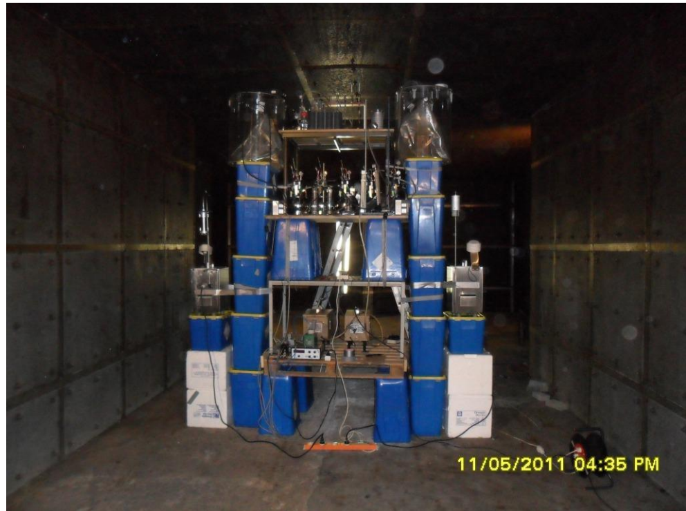
Figure 4 The test set-up 25-100 cm below the ceiling, during the second burn pit experiment
