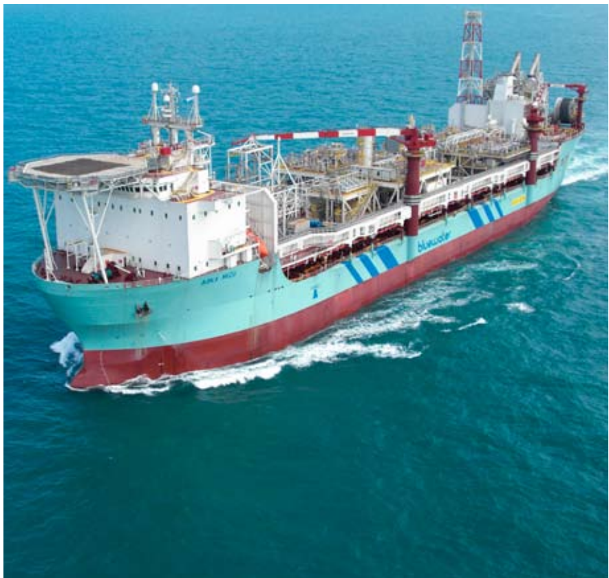
'FPSO Floating Production Storage and Offloading Vessel'
