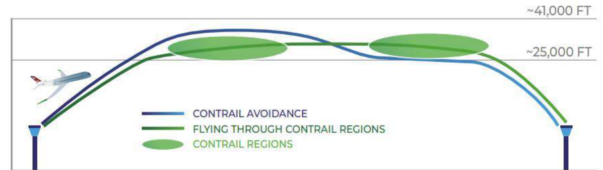
Figure 44 - Schematic representation of navigational contrail avoidance
