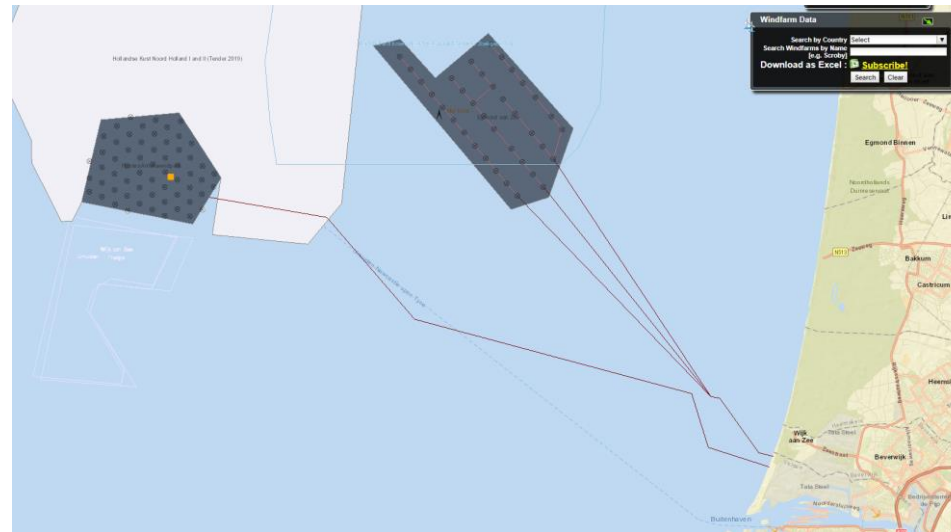
Figure 16. Path of export cables Prinses Amaliawindpark (left) and Offshore Windpark Egmond aan Zee (right).
