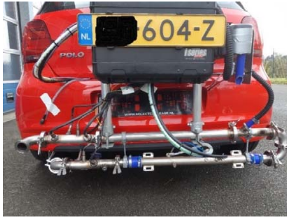
Figure 2-3: Flow measuring tube with dilution air pump and lambda, NO x -O 2 and NH 3 sensors.
