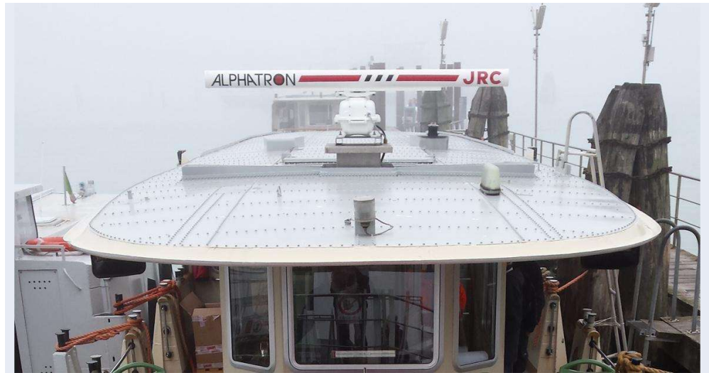
Figure 3-3 JRC JMA-610 radar, note the size as compared to the wheel house (Picture Alphatron Marine)
