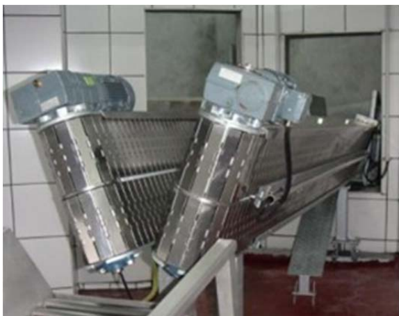
Figure 3: V-shape conveyor belt
