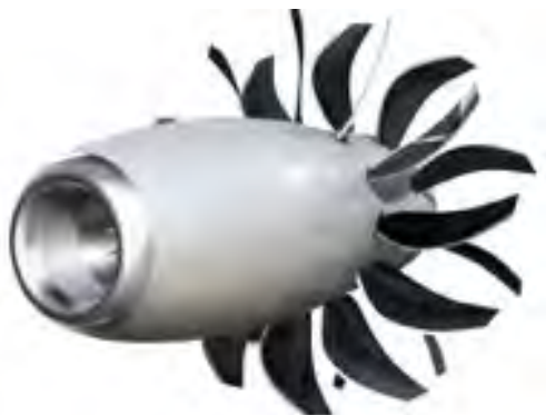
Figuur 7: Open rotor (bron: http://www.cleansky.eu/sustainable-and-green-engines-sage )
