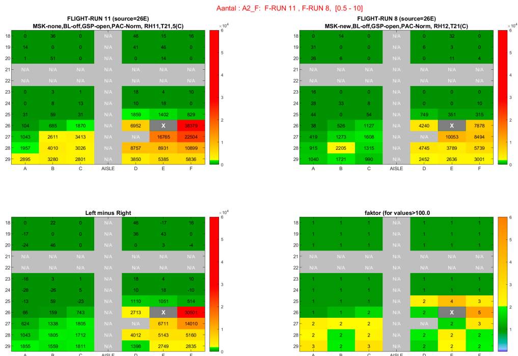
Figure 44: Aerosol distribution with no mask (left) and with mask (right) on index during cruise in B737
