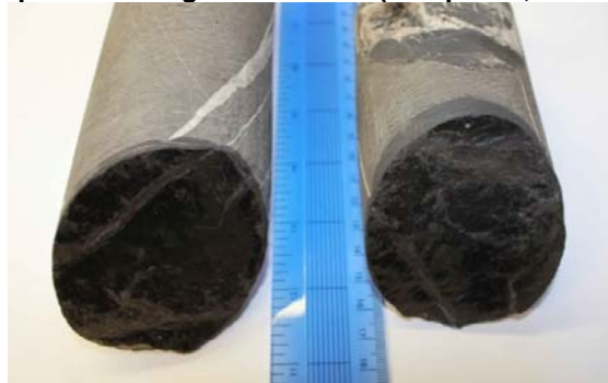
Figure 15: Carbonate siltstone for sliding friction tests (Sample 18; Box 18, 6830.0-6833.1 ftMD)
