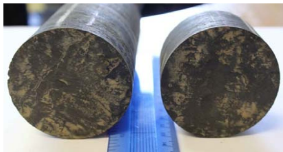
Figure 14: Mudstone sample for sliding friction tests (Sample 13; Box 13, 6813.2-6816.5 ftMD)
