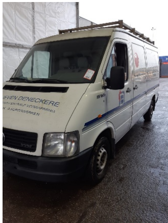
A Volkswagen from 2002 for Tema, Ghana, several deficiencies: light units broken, back door cannot open, oil leak, defective wiper
