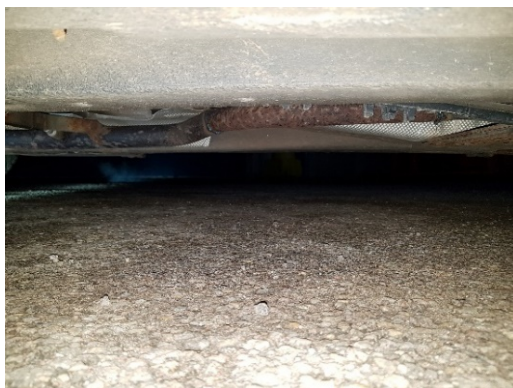
Catalytic converter replaced by a straight exhaust pipe, German BMW from 2001 (left picture) and a German Mercedes C180 from 2000 (right picture) © ILT December 2019
