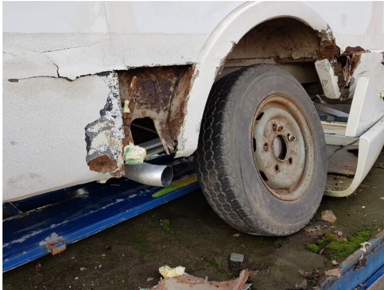
A Volkswagen bus LT3590 from 1988 for Lagos, Nigeria with many damages: left auxiliary beam 100% rust damage, shaft seriously deformed, heavy gasoline smell
