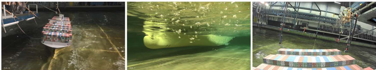
Different views of the tested model of an Ultra Large Container Ship (from MARIN Report 31847-1-SHIPS).
