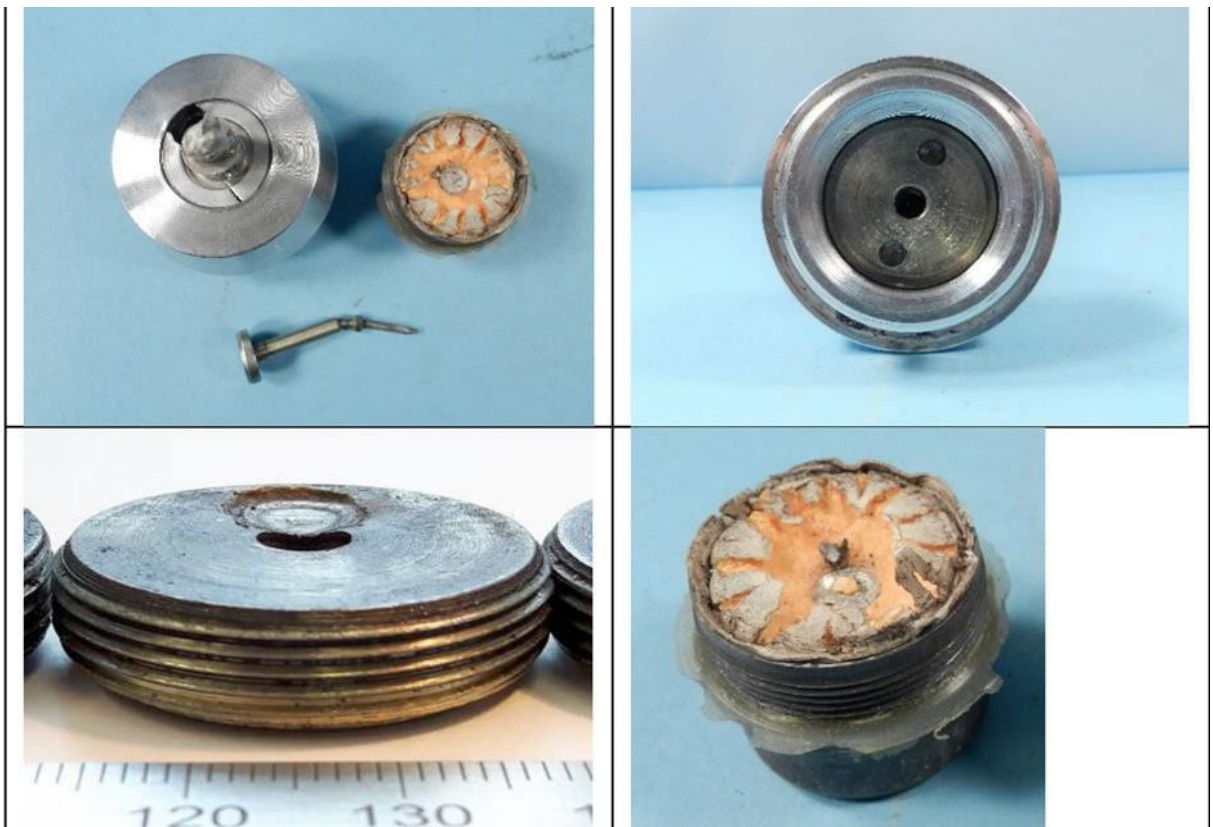
Figure 32: Pictures from TNO Explosives train interruption test, from top left, clockwise: impact fuze after the experiment; bottom surface of the barrier with debris of the lead charge cup; indentation of base of the lead charge cup in the booster charge; impacted interrupter plate with an indentation at the location of the duplex detonator. (Picture: TNO)
