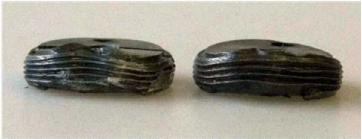
Figure 9: Left explosion train interrupter plate; DSB-report; right explosion train interrupter plate; controlled destruction. (Picture KC W&M)
