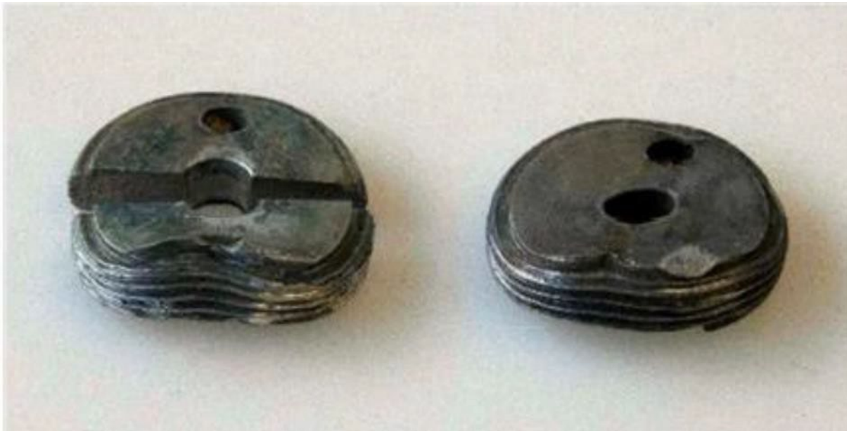
Figure 8: Left explosion train interrupter plate; DSB-report; right explosion train interrupter plate; controlled destruction. (Picture KC W&M)
