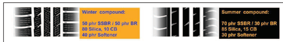
Figure 3.1: Comparison of typical winter and Summer tyre [8].
