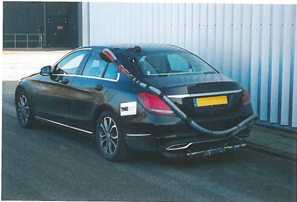
Figure 5: A test vehicle equipped with a Portable Emission Measuring System (PEMS).
